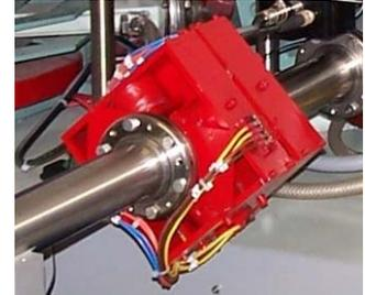
Figure 1. One of the quadrupole focus coil assemblies used in our linear accelerator
